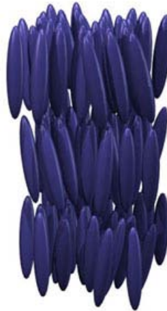
Fig. 1.13 Arrangement of molecules in the smectic-A phase
