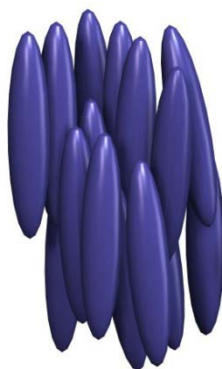
Fig. 1.4 Arrangement of molecules in a liquid crystal
