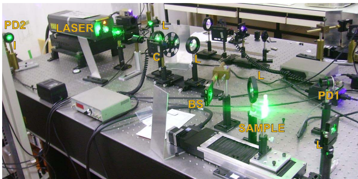
Fig. 3.54 Experimental configuration of Thermal lens in Z-scan technique
