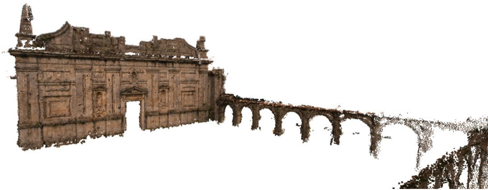
Figure 1.7. 3D point cloud of the Certosa of Serra San Bruno (Italy), destroyed in 1783 by a terrible earthquake.
