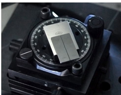
Figure 2.7. Two certified gauge blocks are placed on a rectified surface and mounted on the rotational stage in order to verify the accuracy.
