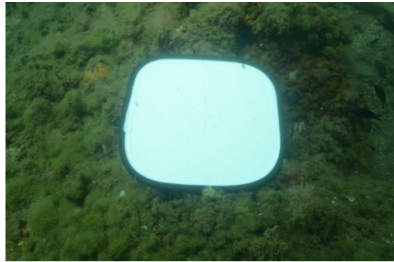
Figure 4.2. Calibration panel used to manually correct the white balance.
