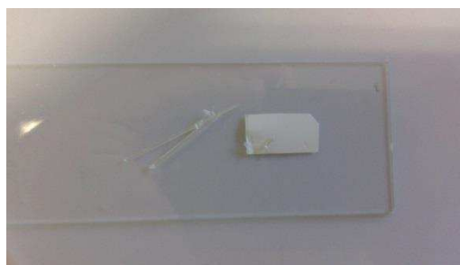
Figure 4. Pictures of INA crystals grown at 1.8 supersaturation in presence of PP7
