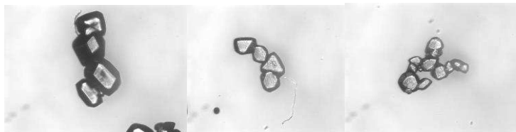
Figure 9. Optical microscope pictures of ACM crystals in batch solution at 16,99 g/L crystallized on PP membrane. These crystals supposedly detached by the membrane surface during the growth.
