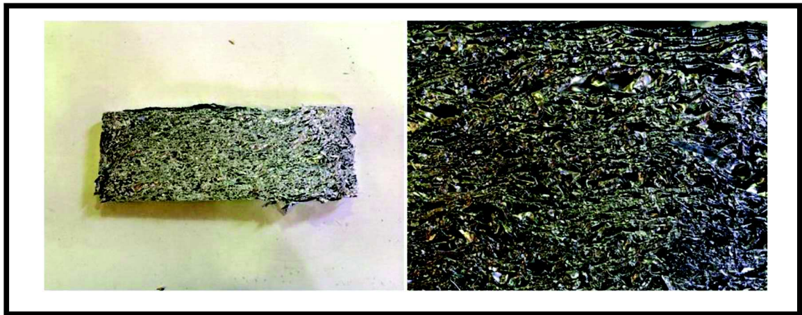
Fig. 5.4: Cold compaction result in Alupack LTD
