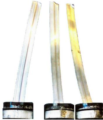
Figure 1.37. Comparison of the Profile 2 curvature, when applying a flat die (on the left), an intermediate pocket (in the middle) and a bigger pocket (on the right), [48]
