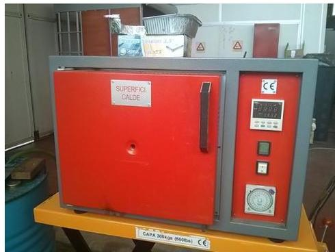
Figure 2.30. Electrical furnace
