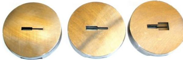
Figure 1.34. Three pocket designs for Profile 1, [48]
