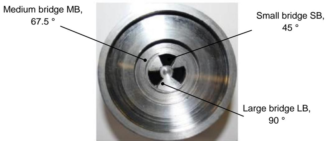
Figure 3.5. Porthole die with different bridges
