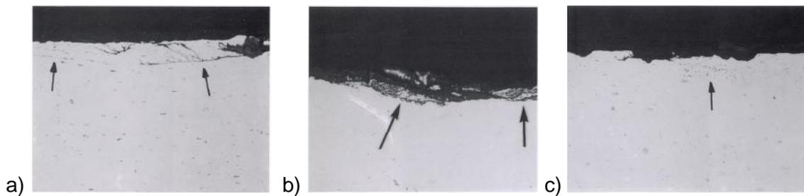
Figure 2.17. Streaks defect microstructure (500x) on an orthogonal plan to the defected surface, [100]
