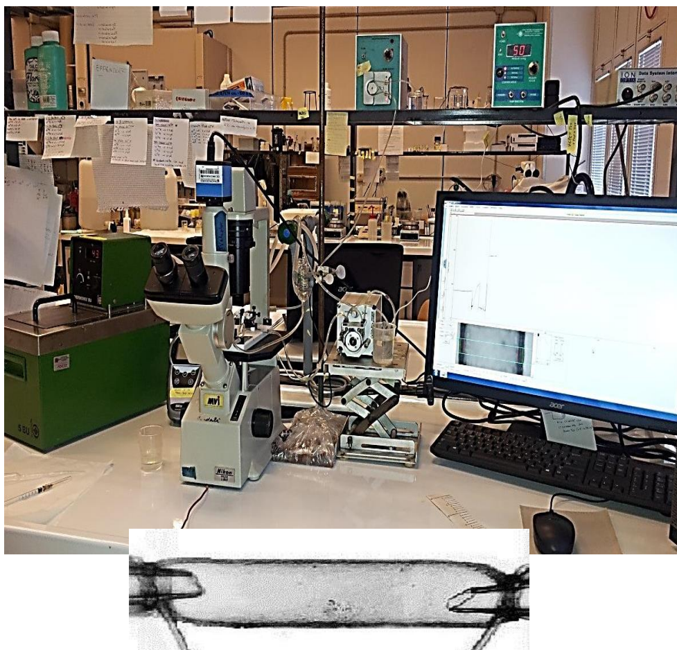
Figura 15: Pressure myography e arteria incannulata.
