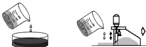
Scheme 2. Casting Procedures Followed in Order to Prepare Membranes: Casting in a Petridish (left) and Spread with a Knife (right)
