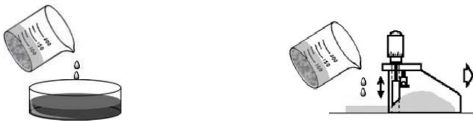
Figure 13. Casting procedures followed in order to prepare membranes: casting in a petridish (left) and spread with a knife (right).
