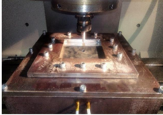
FIGURE 3.24 DRILLED ALUMINIUM SHEET LAID ON THE COMPOSITE ONE
