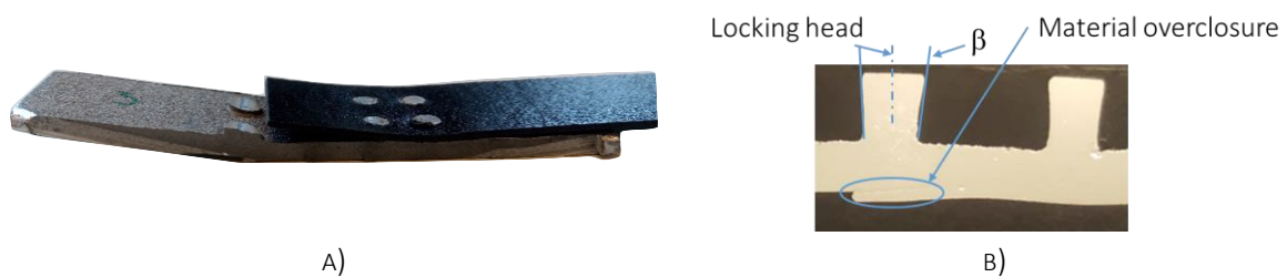
FIGURE 4.22 A) EXAMPLE OF A PERFORMED JOINT AND B) PIN GEOMETRY AFTER JOINING
