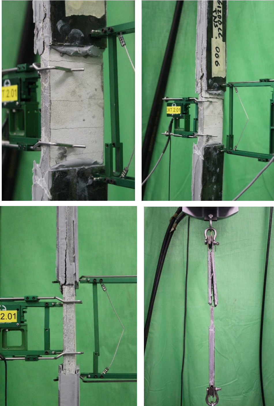
Figure 6.12 – Representative failure mode of coupons GLT-G12 subject to tensile test
