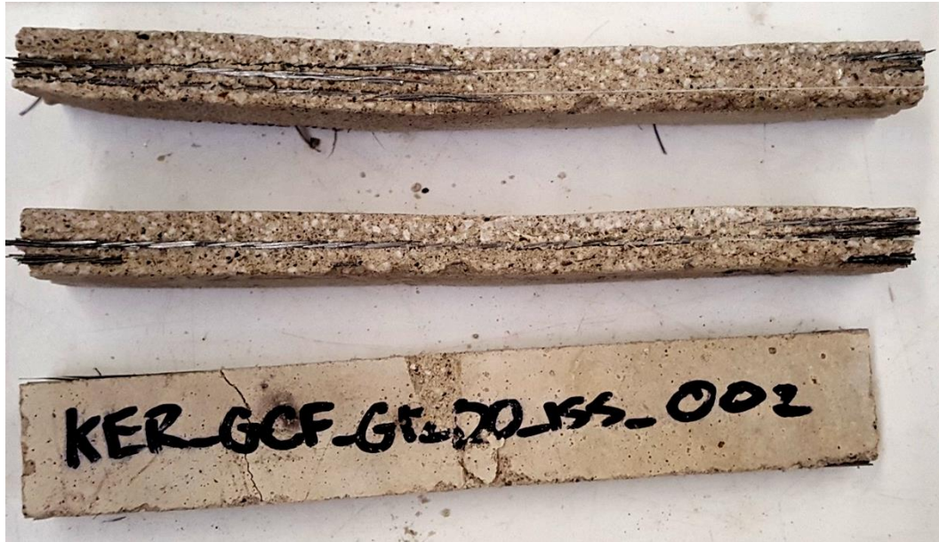
Figure 7.6 - Failure mode of the specimens GCF-G12-2
