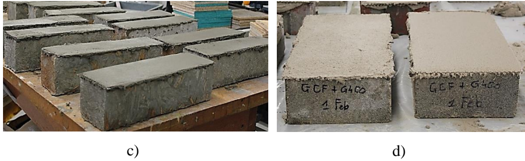
Figure 8.3 - Specimens preparation: a) Cleaning of specimens by any debris, b) Reinforcement applied on clay bricks, c) Reinforced concrete blocks and d) Reinforced concrete masonry units
