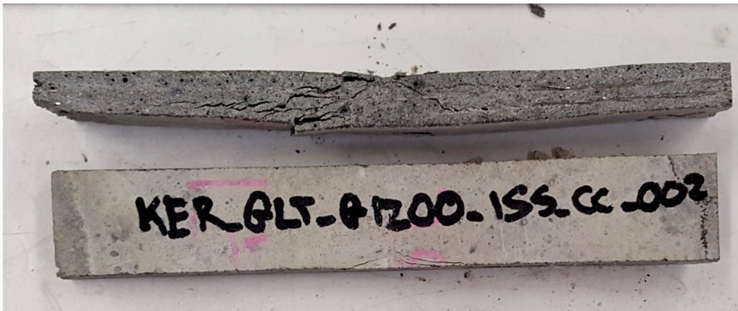
Figure 7.8 - Failure mode of the specimen GLT-G12-2
