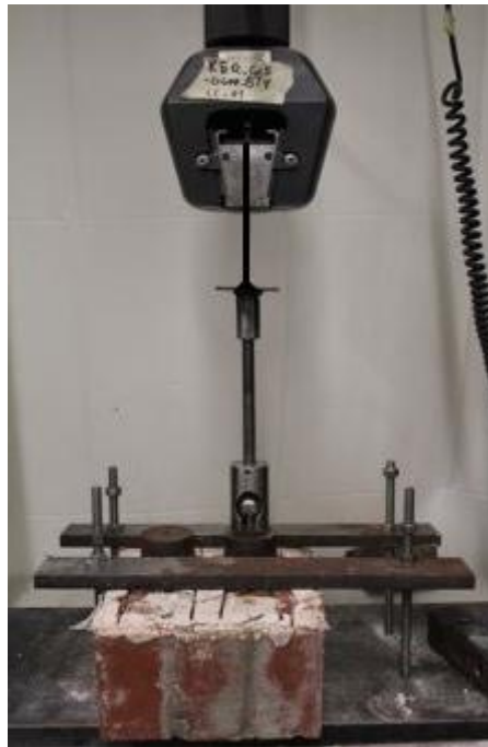
Figure 8.5 - Pull-off test set-up
