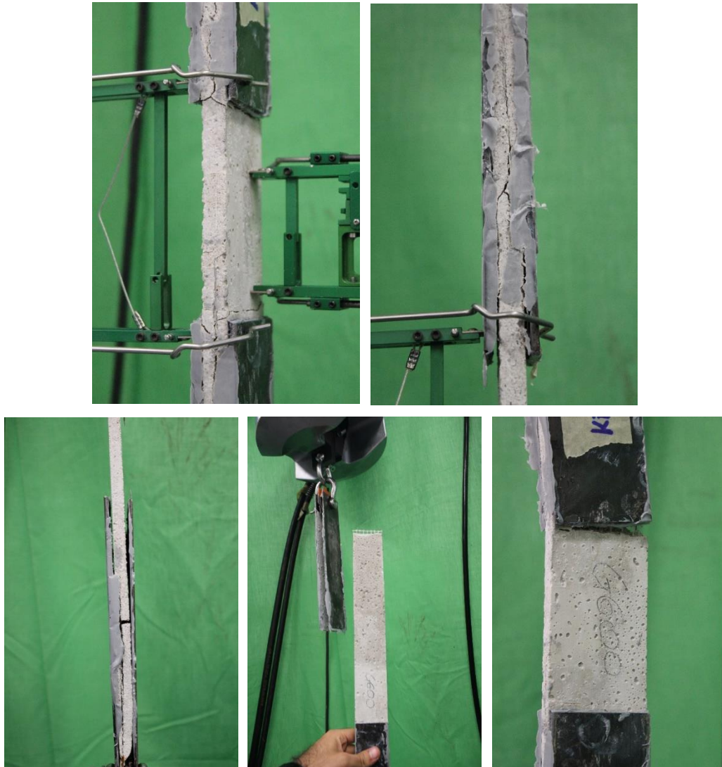
Figure 6.14 - Representative failure mode of coupons GCF-G6 subject to tensile test
