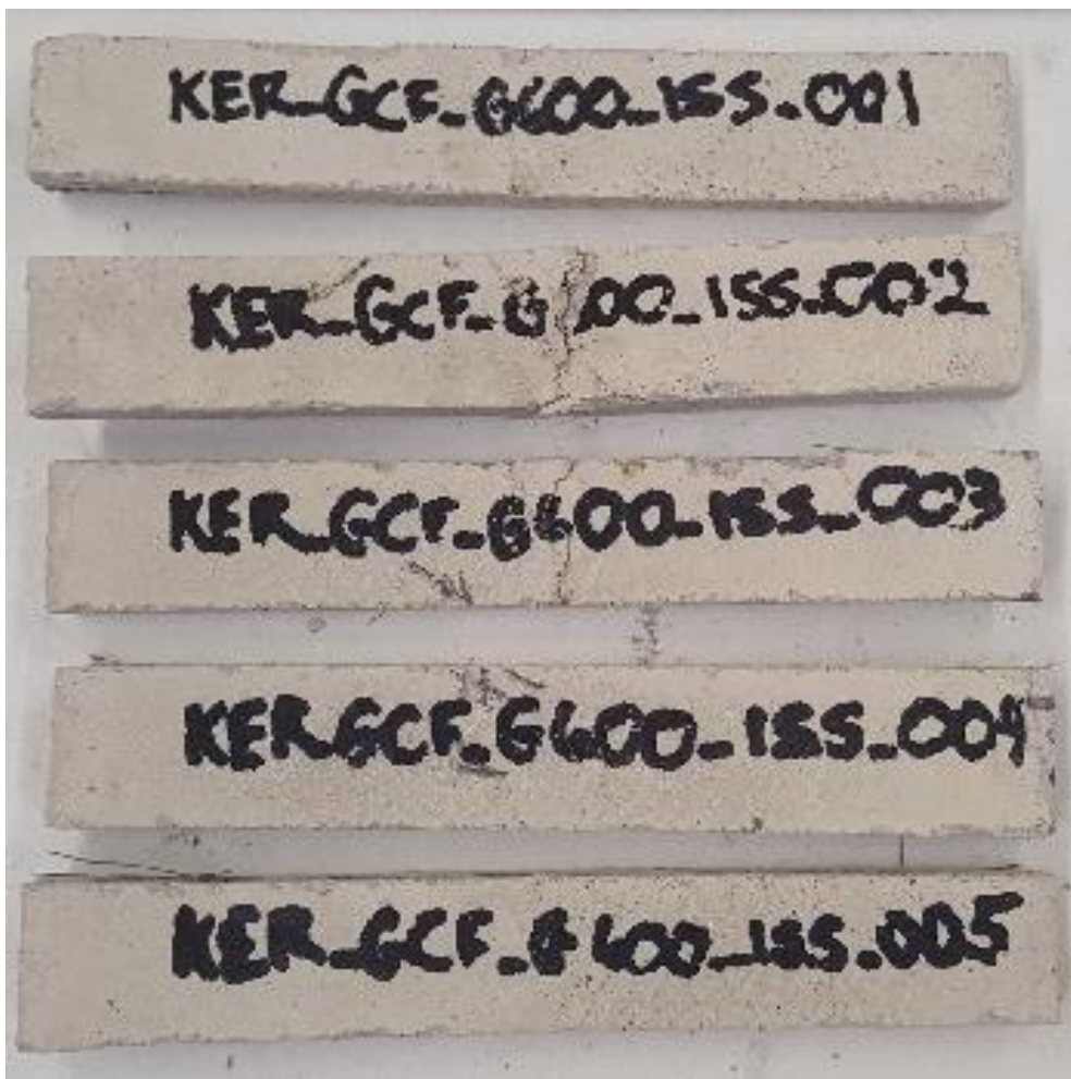
Figure 7.5 - Failure modes of the GCF-G6 specimens
