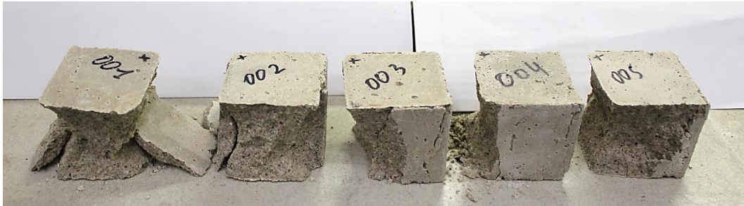
Figure 5.8 - Failure modes of cubes made of GCF at curing time of twenty-eight days
