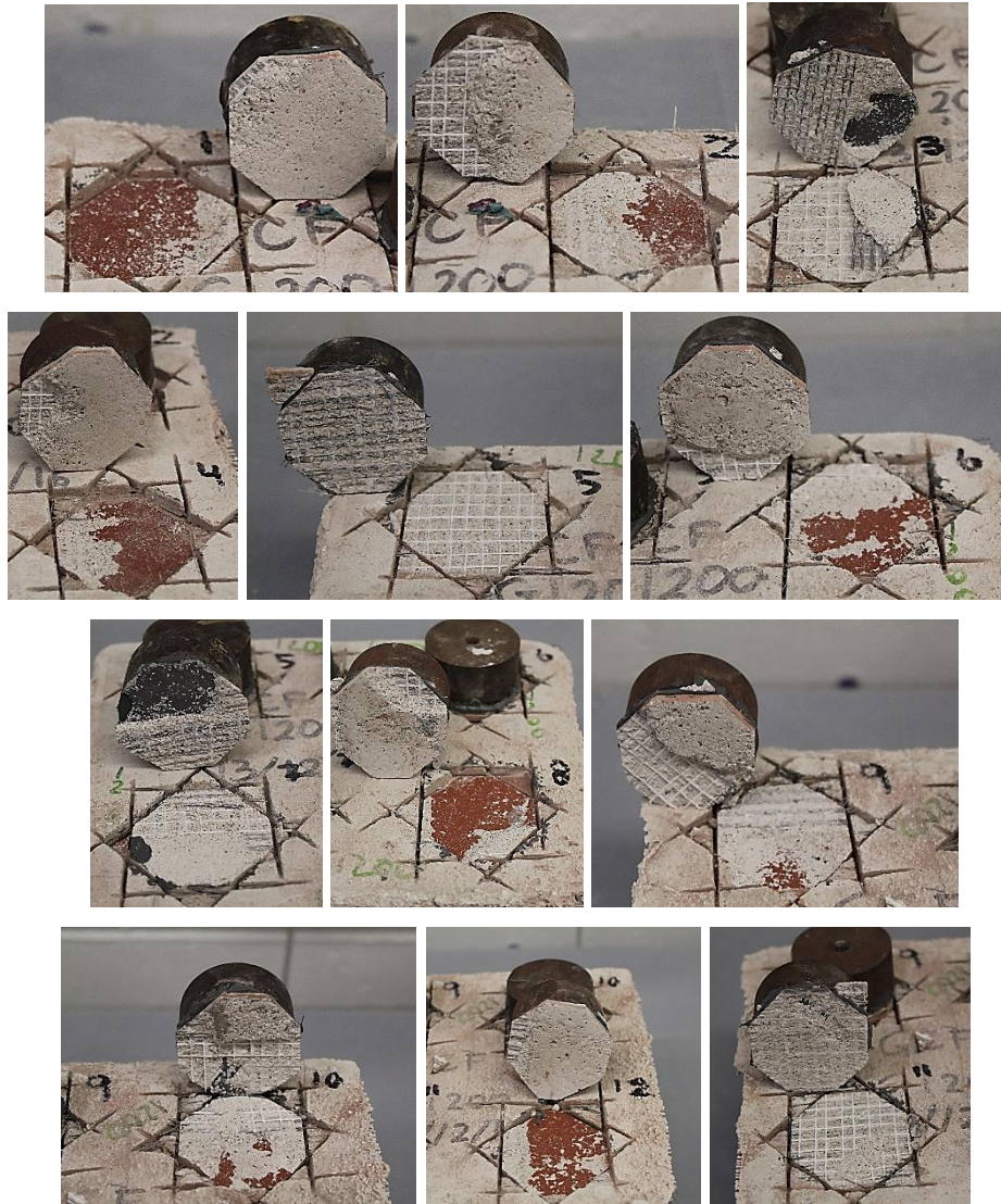
Figure 8.8 -Failure modes of the BTY-GCF-G12 series
