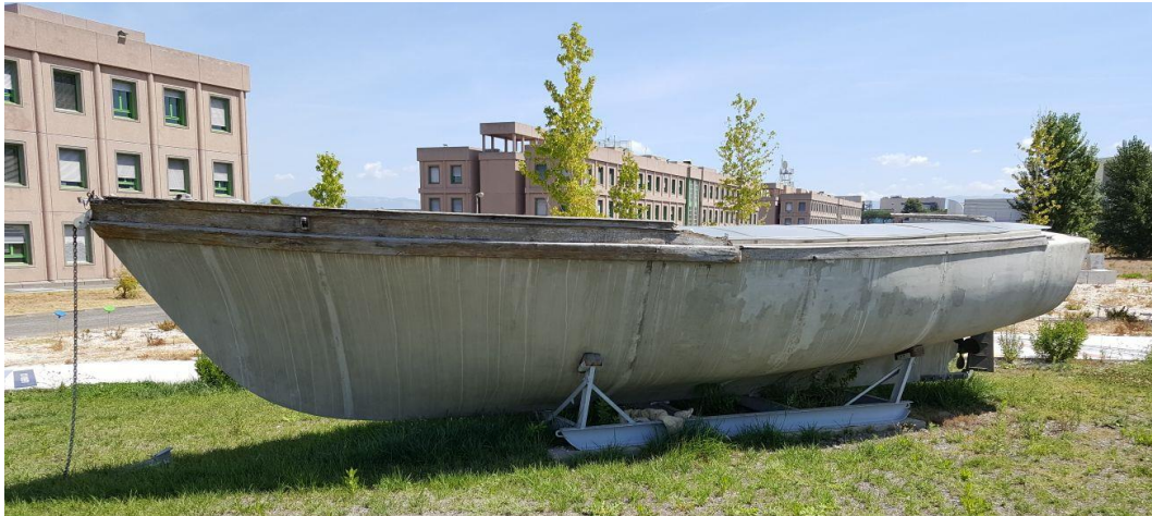
Figure 1.5 - Ferrocement boat hull built by Nervi, 1972
