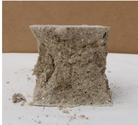
Figure 5.6 - Representative failure modes of cubes made of GCF at curing time of seven days
