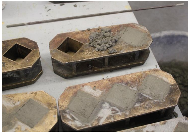
Figure 5.1 - Cube molding for compressive strength of mortar tests
