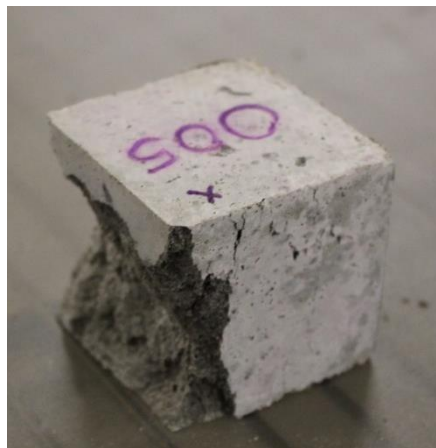
Figure 5.12 - Representative failure modes of cubes made of GLT at curing time of twenty-eight days
