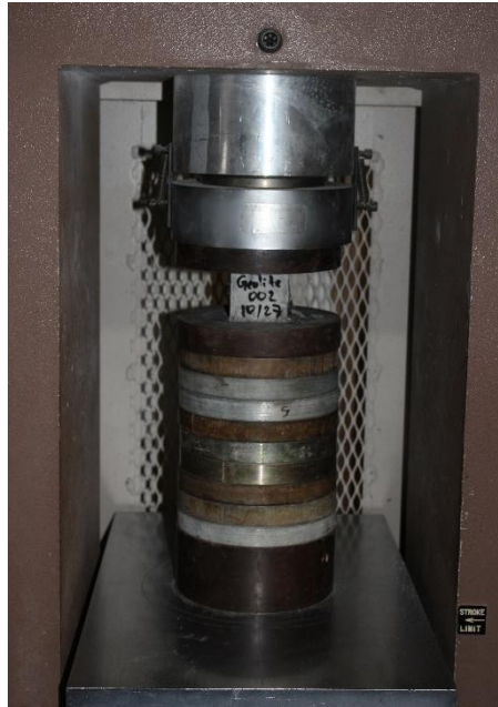
Figure 5.3 - Compressive test set-up
