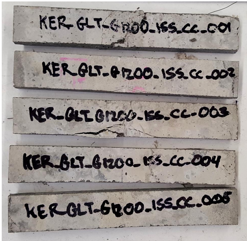
Figure 7.9 - Failure modes of the GLT-G12 specimens
