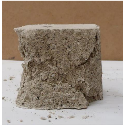
Figure 5.7 - Representative failure modes of cubes made of GCF at curing time of fourteen days
