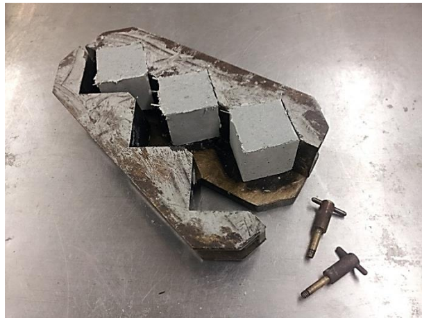
Figure 5.2 - Cube de-molding for compressive strength of mortar tests
