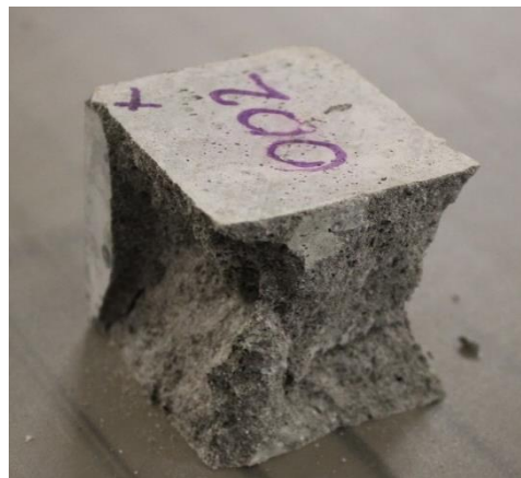
Figure 5.10 - Representative failure modes of cubes made of GLT at curing time of seven days
