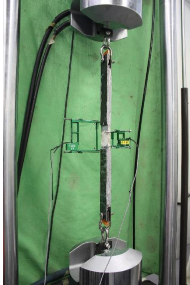
Figure 6.6 - Tensile test set-up
