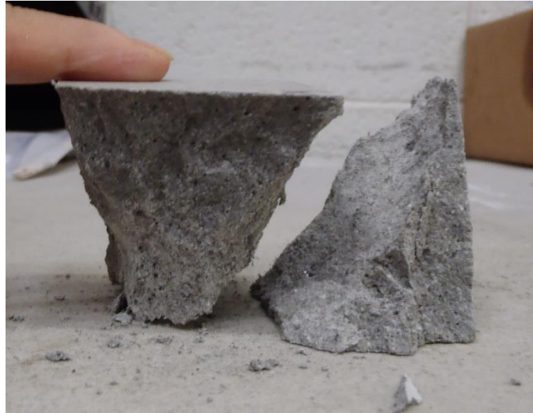
Figure 5.9 - Representative failure modes of cubes made of GLT at curing time of three days
