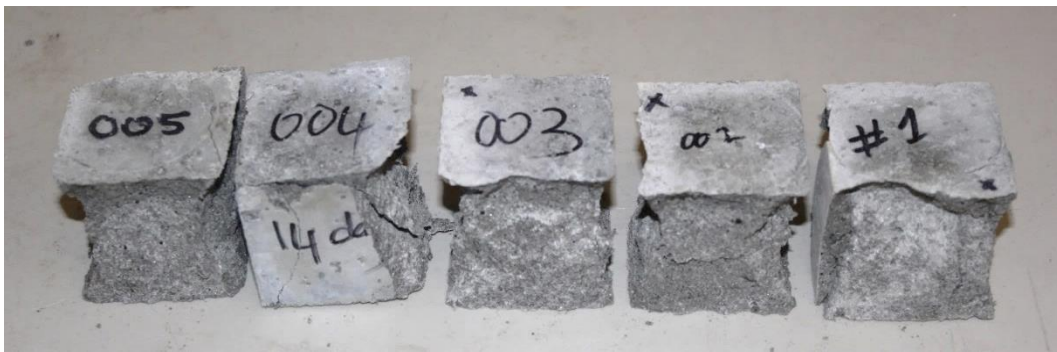
Figure 5.11 - Failure modes of cubes made of GLT at curing time of fourteen days
