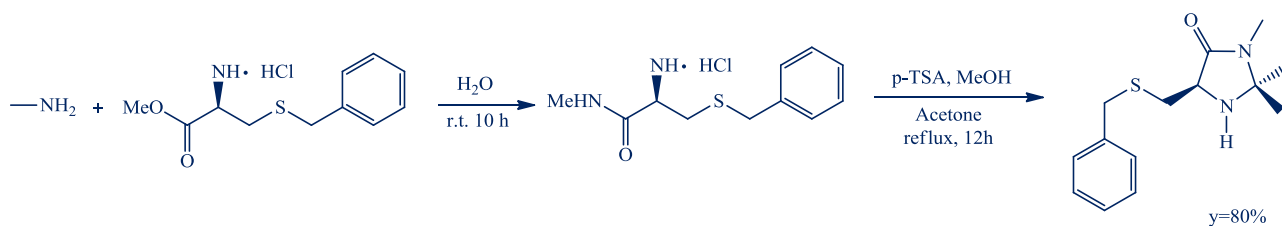
Scheme 10.2 Synthesis of (5 S )-2,2,3-trimethyl-5-thiobenzylmethyl-4-imidazolidinone.
