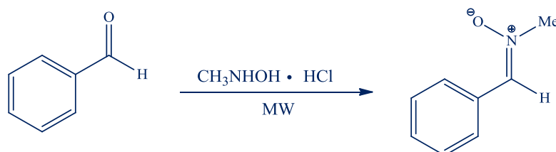
Scheme 8.2 Model reaction to synthesize nitrones.
