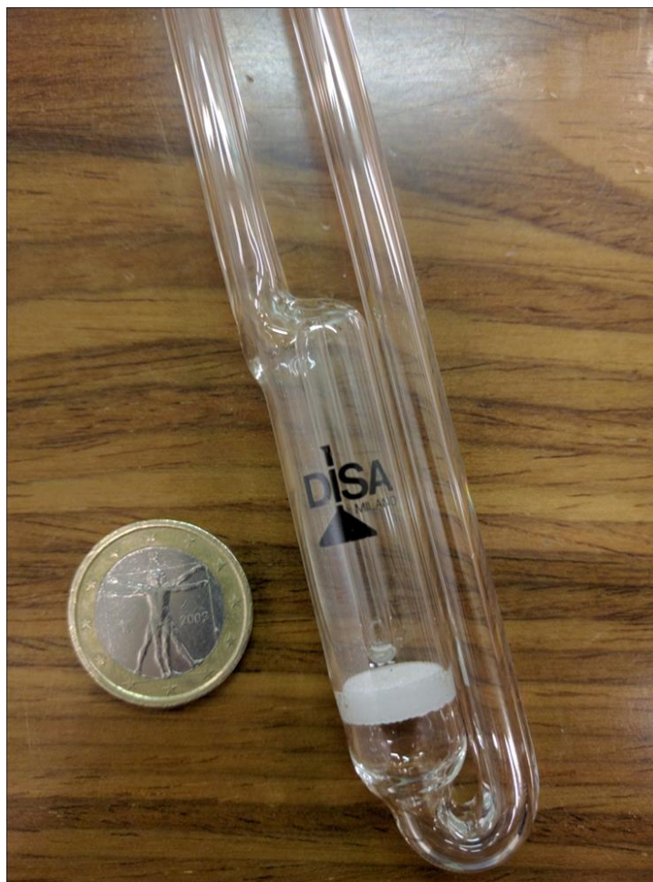
Figure 3.2 – Reactor used for methanol conversion reaction
