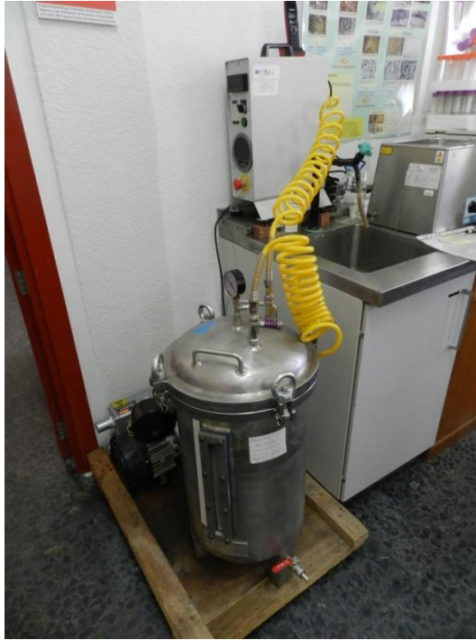
Fig. 5.10. Evacuation vessel employed for the water absorption by total immersion test under vacuum.
