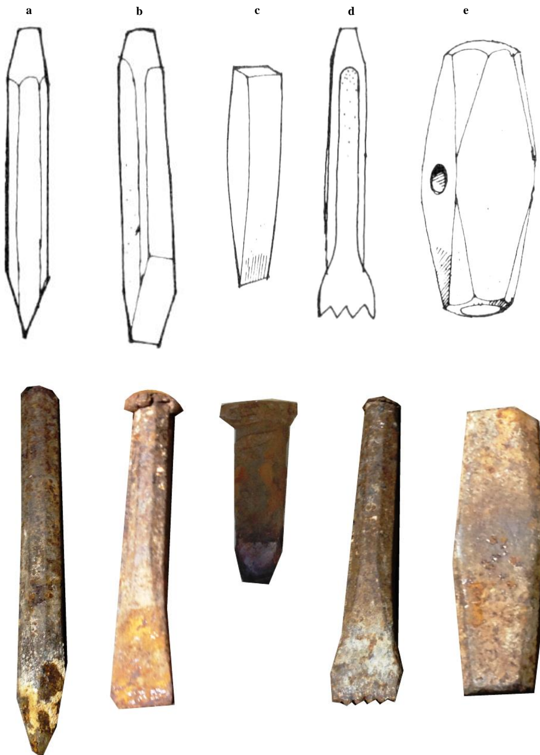
Fig. 3.32. Splitting devices: point chisel (a); standard chisel called “pungiotto” (b); wedge (c); toothed chisel (d); striking-hammer (e). Hammers and chisels employed by the stonemason Silvio Ferrari, belonging to the school of stonemasons of Altilia.
