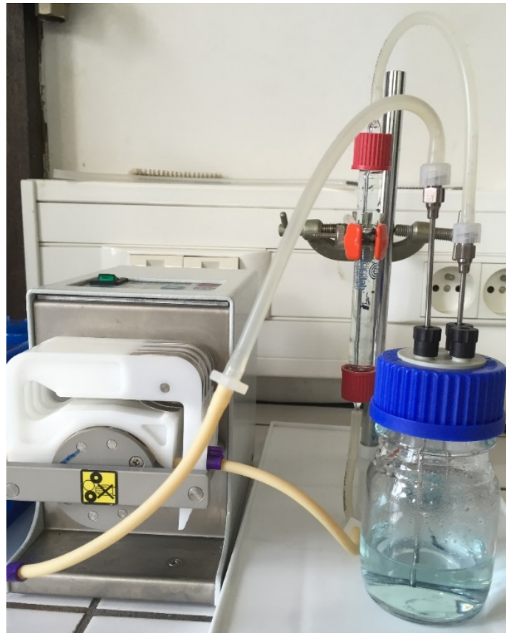
Figure 8. 3 Fluidized bed bioreactor using (cell-free) alginate beads, expansion ratio 2 ( h_i=5\text{cm} ), flow rate 1.4 ml/min
