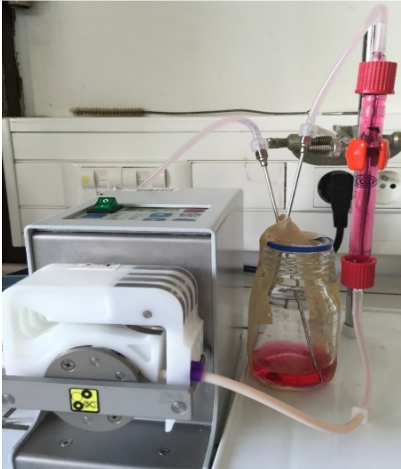
Figure 8. 5 Fluidized bed bioreactor used to study the transport of vitamin B12 into the beads (dynamic system)
