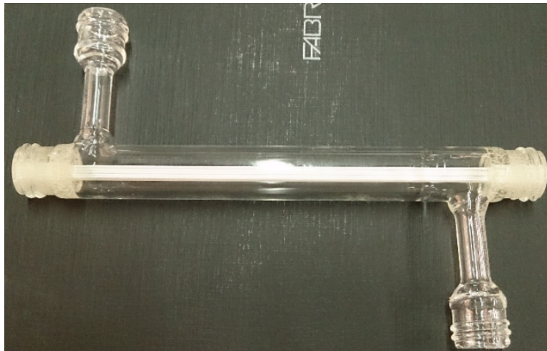
Figure 2. 1 Hollow fiber module assembled for permeability measurements (25 PEEK-WC hollow fibers, 5x5 arrangement).
