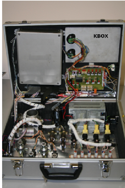
Figure 7.2 The MHIL hardware components: a console containing the actuators (external loads), the ECU under test and the signals generator (KBOX).
