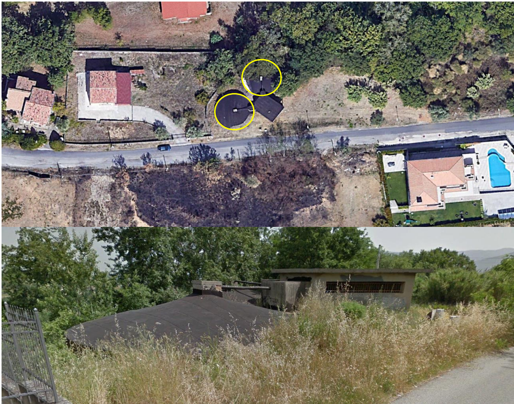
Figure 3.2.4 Ceep/Monello tank characteristic surveying. The tank has two circular storage compartments partially buried. The figure shows a tank plan view (Google Earth).
