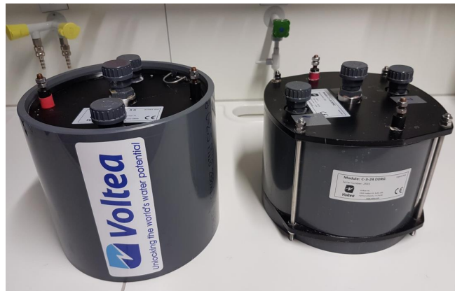
Figure 6.2. Two C-3 MCDI modules from Voltea . Left: old design, right: new design
