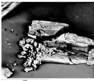
Fig 4.7 SEM image of a crystal of CU Synthesized C 6 H (Magnification: 50x)
