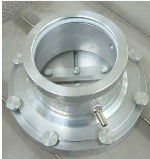
**Fig. 2:** Shielding chamber
