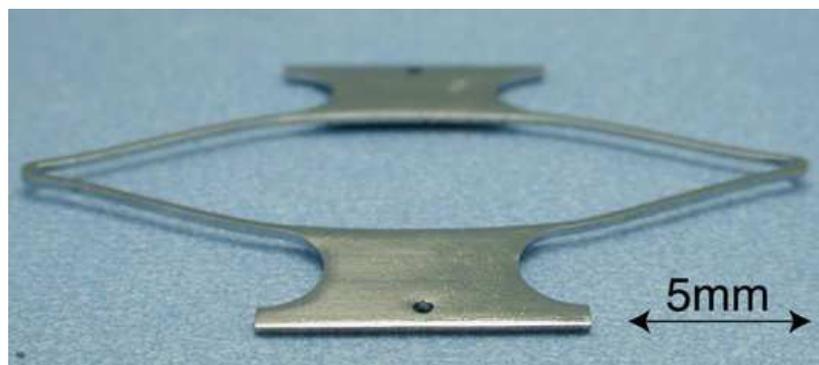
**Figure 2.4:** NiTi diamond shaped specimen [84].
