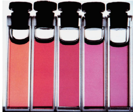
Figure 2-10 plasmon peak position variation induced by changing the solvent refractive index. Refractive indices of the solutions at the absorption band maximum are 1.336, 1.407, 1.481, 1.525 and 1.583, respectively [36].
