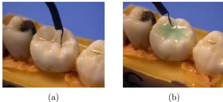
Figure 2.5: Electrical Caries Monitor: (a) site-specific and (b) surface-specific measurement modes.
