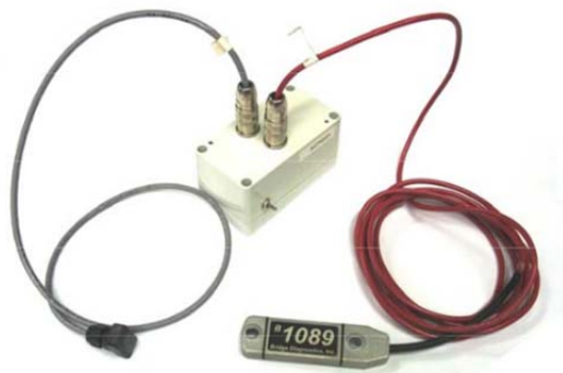
Fig. 3.9 – Wireless Sensing Solution proposed by Whelan (source: Whelan and Janoyan [102])
