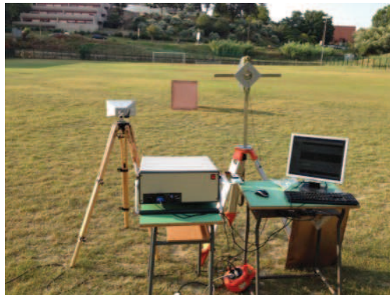
Fig. 1.30. Photograph of the L-band SDRadar system during the outdoor experimentation.
