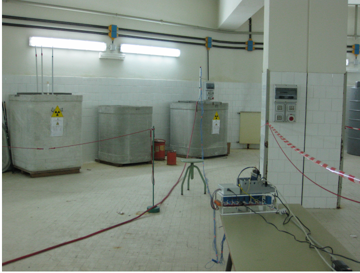
Figure 2.16: Capacitor and DUT boards arrangement into the irradiation room at the UniPA neutron facility
