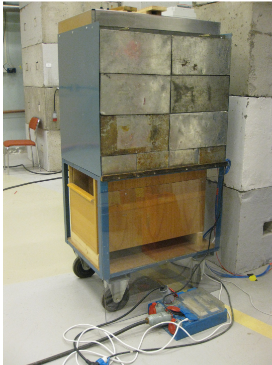
Figure 2.15: Instrument and capacitor board protection with borated wax bricks at the ANITA facility
