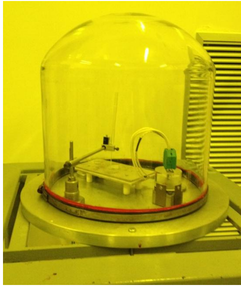
Fig. 3.7.3.1 Filling process in a vacuum chamber
