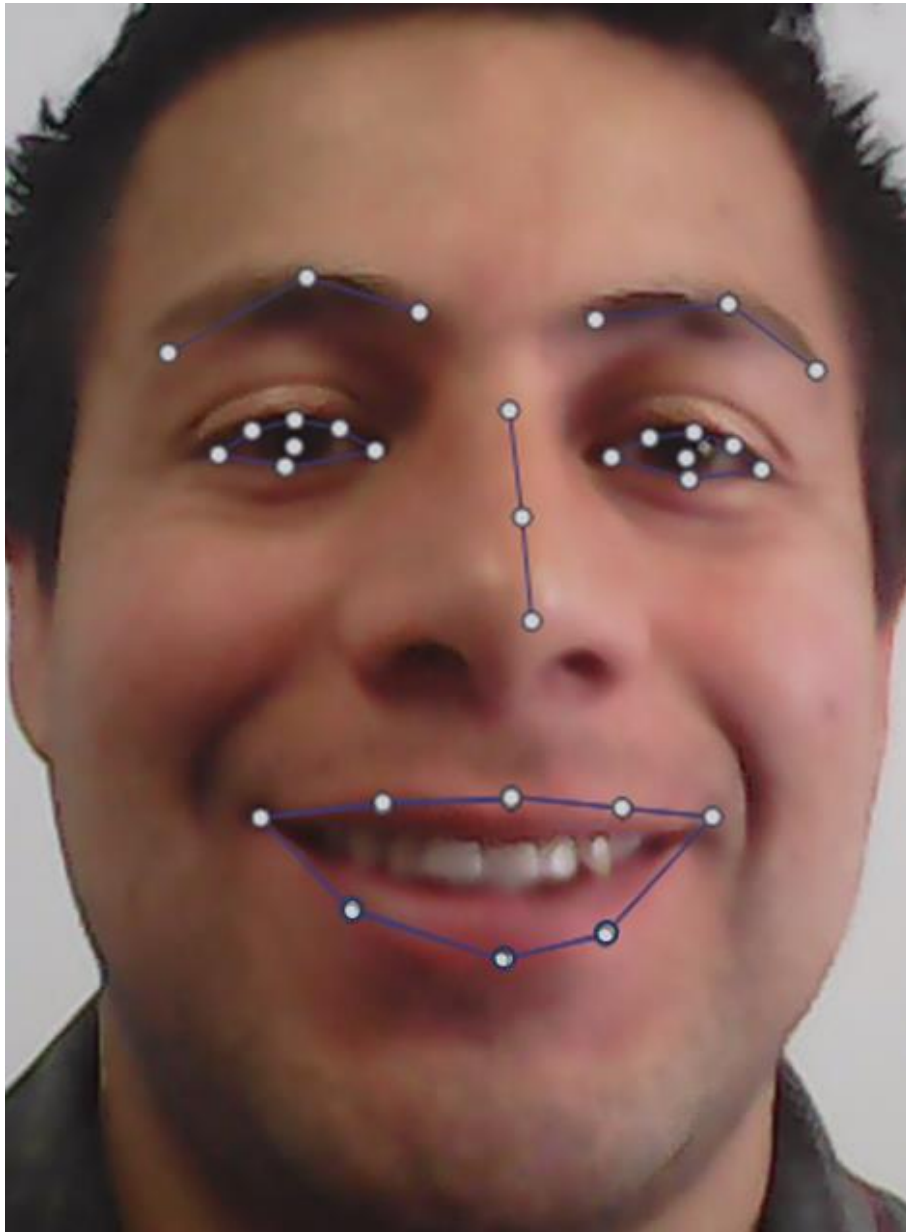
Figure 34. Face Land Marks provided by NAO's ALFaceDetection module.
