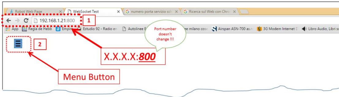
Figure 15. Control interface access. (1) NAO Robot's IP address and port and (2) Web control interface Menu Button.
