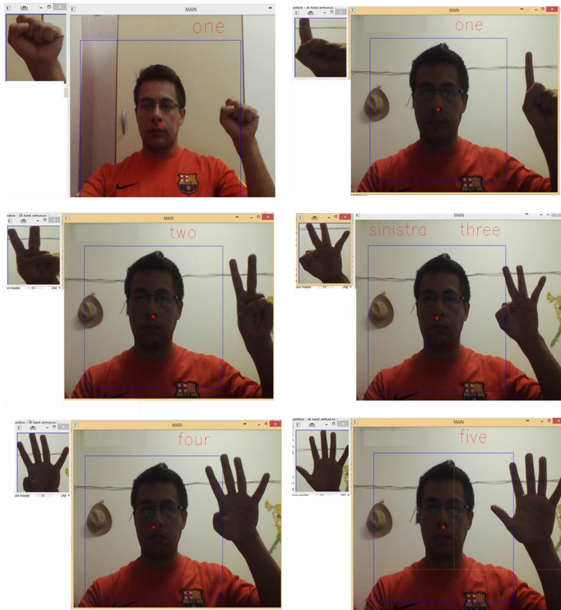
Figure 48. Gesture recognition test using one hand. Most of false positives occurred when recognizing the 0 and 1.
