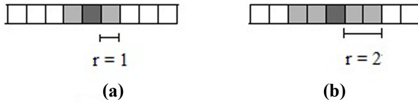
Fig. 2.2 Example of neighborhood with a range of (a) r = 1 and (b) r = 2 for a 1-dimensional cellular automata. The dark gray cells are the central cell, the light gray cells are the neighbors
