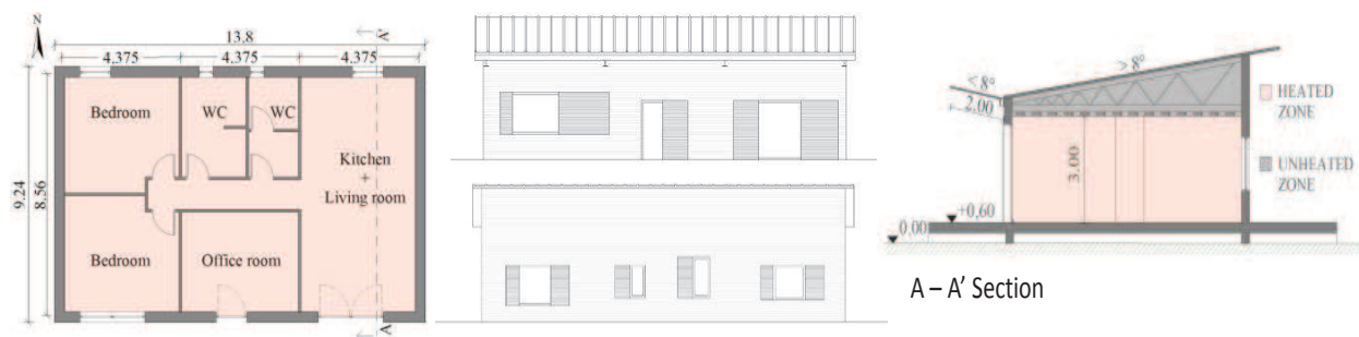
Fig. 5. The reference building considered for energy evaluations.
