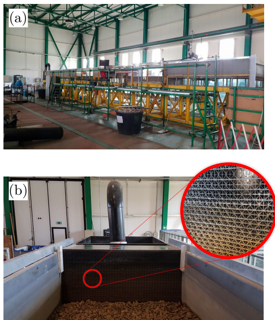
Figure 3.1: Flume details; (a) picture of the installation; (b) honeycomb and details of the triangular pipes.
