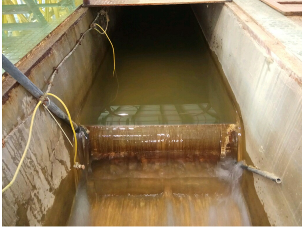
Figure 3.2: Bazin weir used to measure the discharge.
