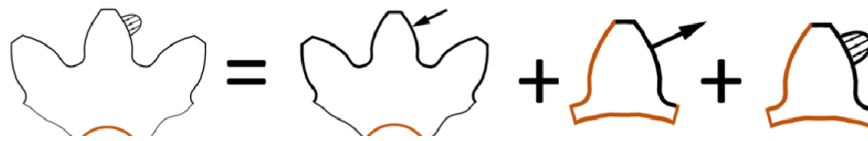
FIGURE 4.2: Computational steps to represent gear total deformation [22].
