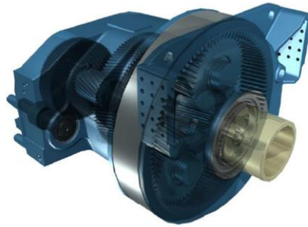
FIGURE 2.20: General Electric 1P 2.3 wind turbine transmission, having one planetary stage and two conventional parallel helical stages. Reproduced from [43]
