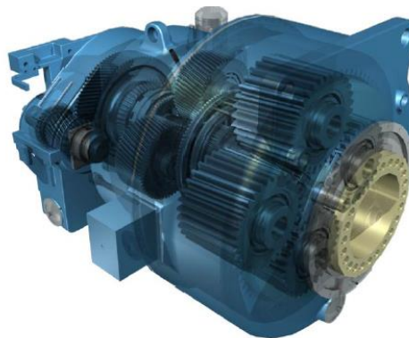
FIGURE 2.21: General Electric 2P 2.9 wind turbine transmission, having two planetary stages and one conventional parallel helical stage. Reproduced from [43].
