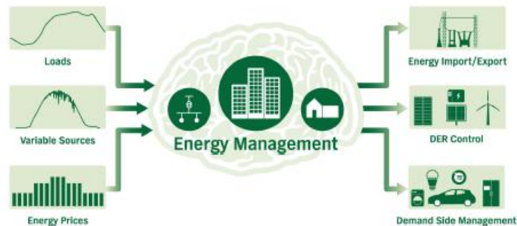
Fig. 2-1 Inputs and outputs of a MG Energy Management System
