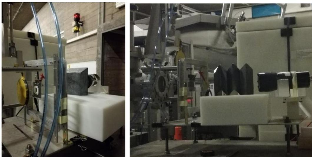
**Figure 5.6:** Figures shows experimental setup with lead bricks placed between the target and the neutron counter.
