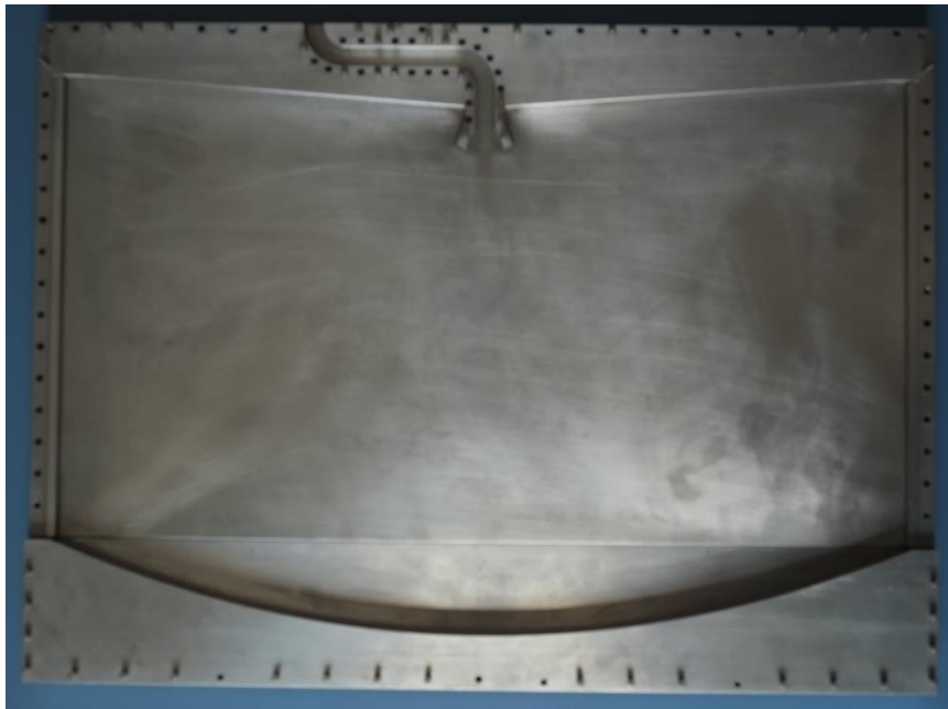
Fig. 3.27 - Feeding structure of the realized antenna
