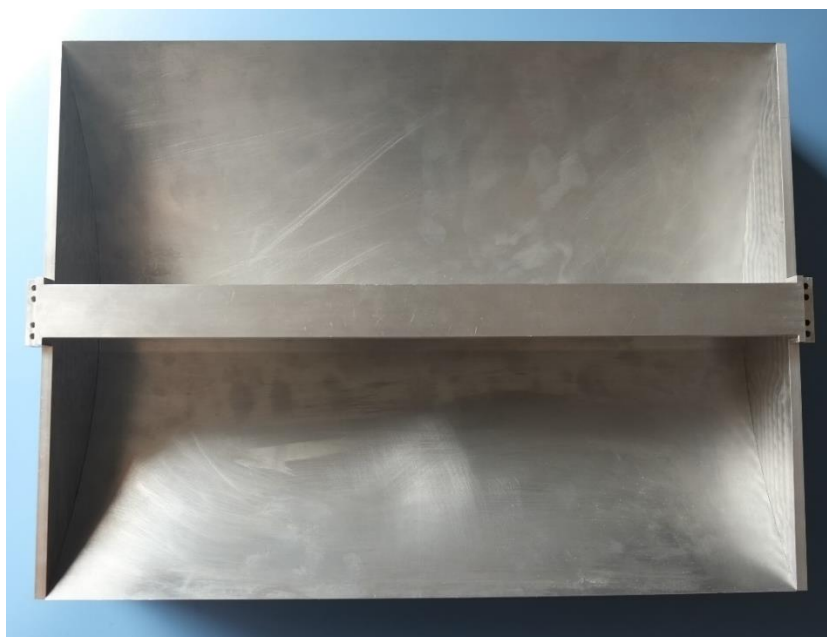
Fig. 3.26 - Top view of the realized antenna in Ka band
