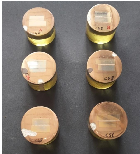
Figure 1.7: cold-mounted and polished cross sections prepared for the microstructural analysis and the indentation tests.
