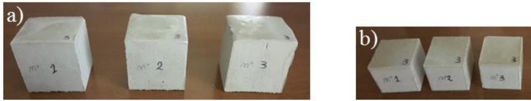
Figure 2.8: cubic samples of dimension a) 40 mm and b) 20 mm produced for the piezoresistive and piezoelectric characterization respectively.
