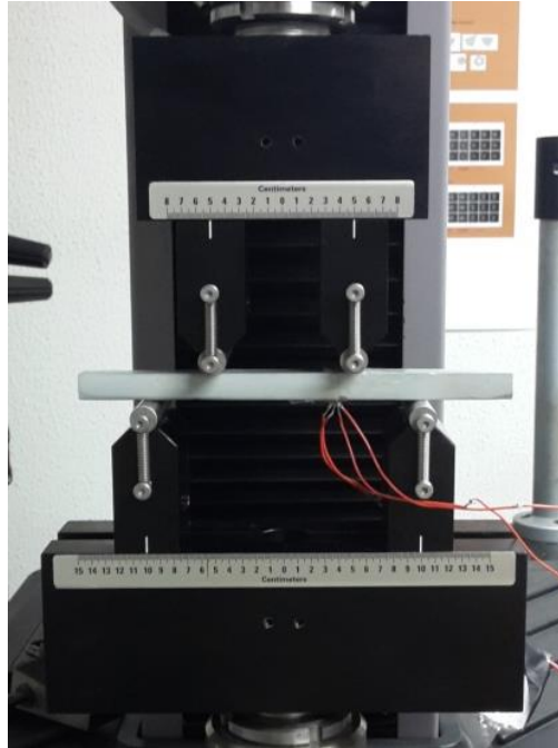
Figure 2.18: experimental setup for the four points bending tests. The red wires connect the XY strain gauge to the Strain Gauge Bridge Amplifier in order to record the strain signal.
