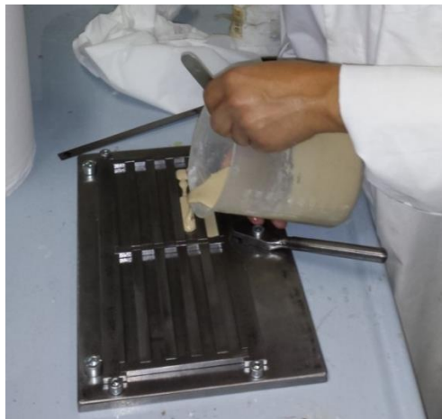
Figure 2.6: casting of geopolymeric mortar into open and dismountable molds.
