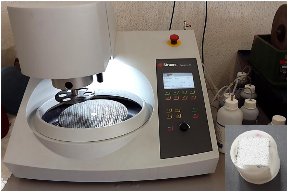
Figure 2.19: Equipment used for the grinding and polishing of geopolymer samples. The inset shows the cold mounted and polished sample.
