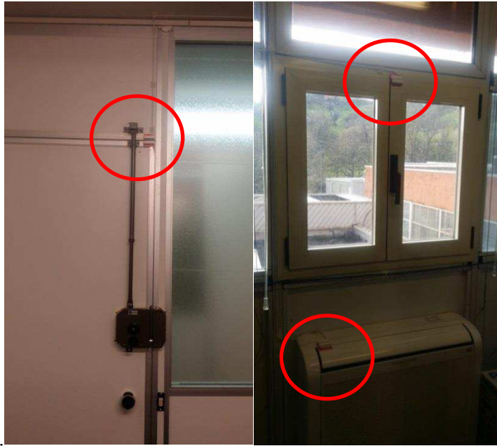
Figure 4.16 Reed switch to measure the window, door position and on/off air conditioner Technical specifications
