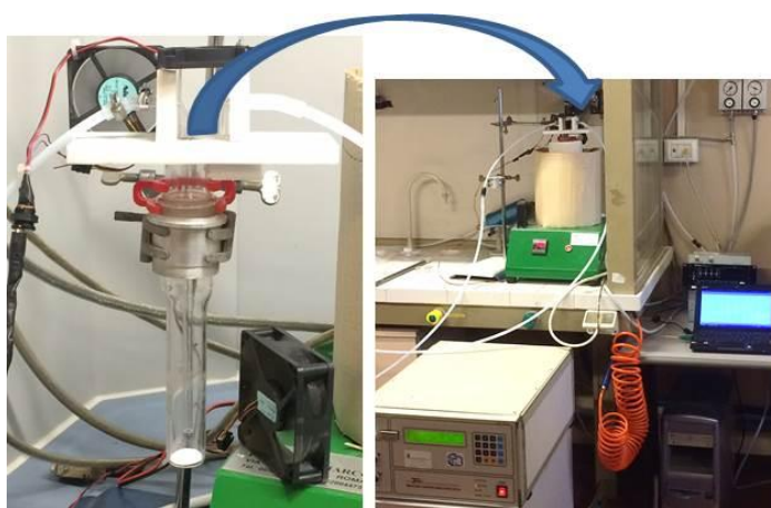
Figure 8.6. CNR-IIA equipment to thermally desorb Hg from passive samplers (quartz tube on the left ), furnace (up to 800°C) and TEKRAN analyzer on the right .
