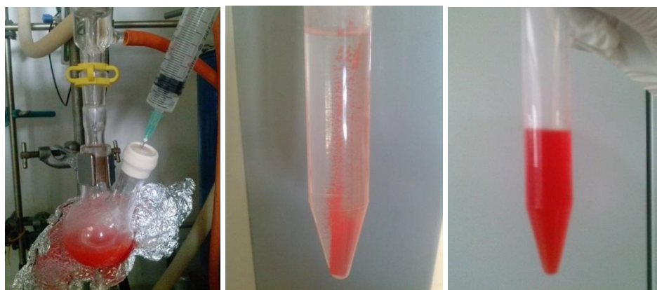
Figure 4.9: Precipitation, centrifugation and dissolution CdSe/ZnS QDs in \text{CHCl}_3
