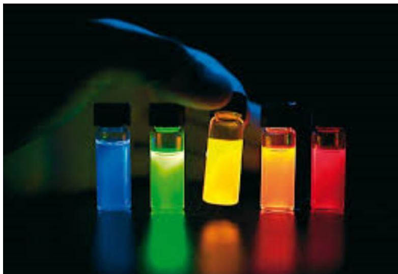
Figure 4.3: Quantum dots of different sizes under excitation from a UV-lamp at 366 nm.
