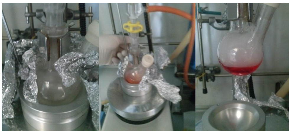
Figure 4.8: Arrest nucleation CdSe core by rapid cooling of reaction after 1.5 minutes.
