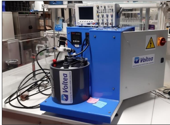
Figure 3.2-1 Lab-scale MCDI (type C5, Voltea®) with a capacity of 0.4-2.6 L/min.
