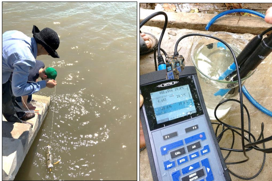
Figure 3.5-1 Sample taking and pH and EC measurements on site (WTW Multi-parameter 3430).
