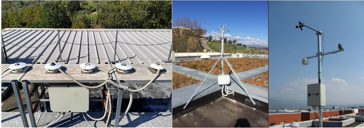
Figure 2. Weather monitoring station for solar radiation on the horizontal plane, external air temperature and wind speed measurement.
