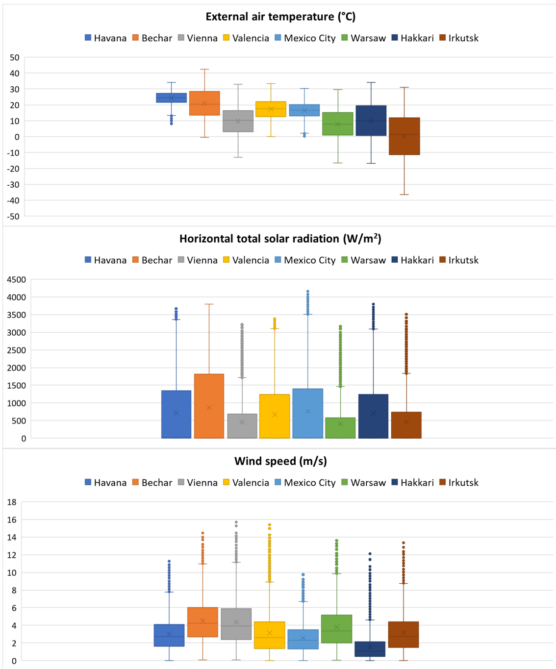
Figure 10. Yearly box plots of the hourly external air temperature, horizontal total solar radiation, and wind speed in the selected locations for the ANN application.
