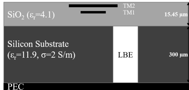
Figure 5-4: Simplified cross-section of IHP SG13S technology with LBE
