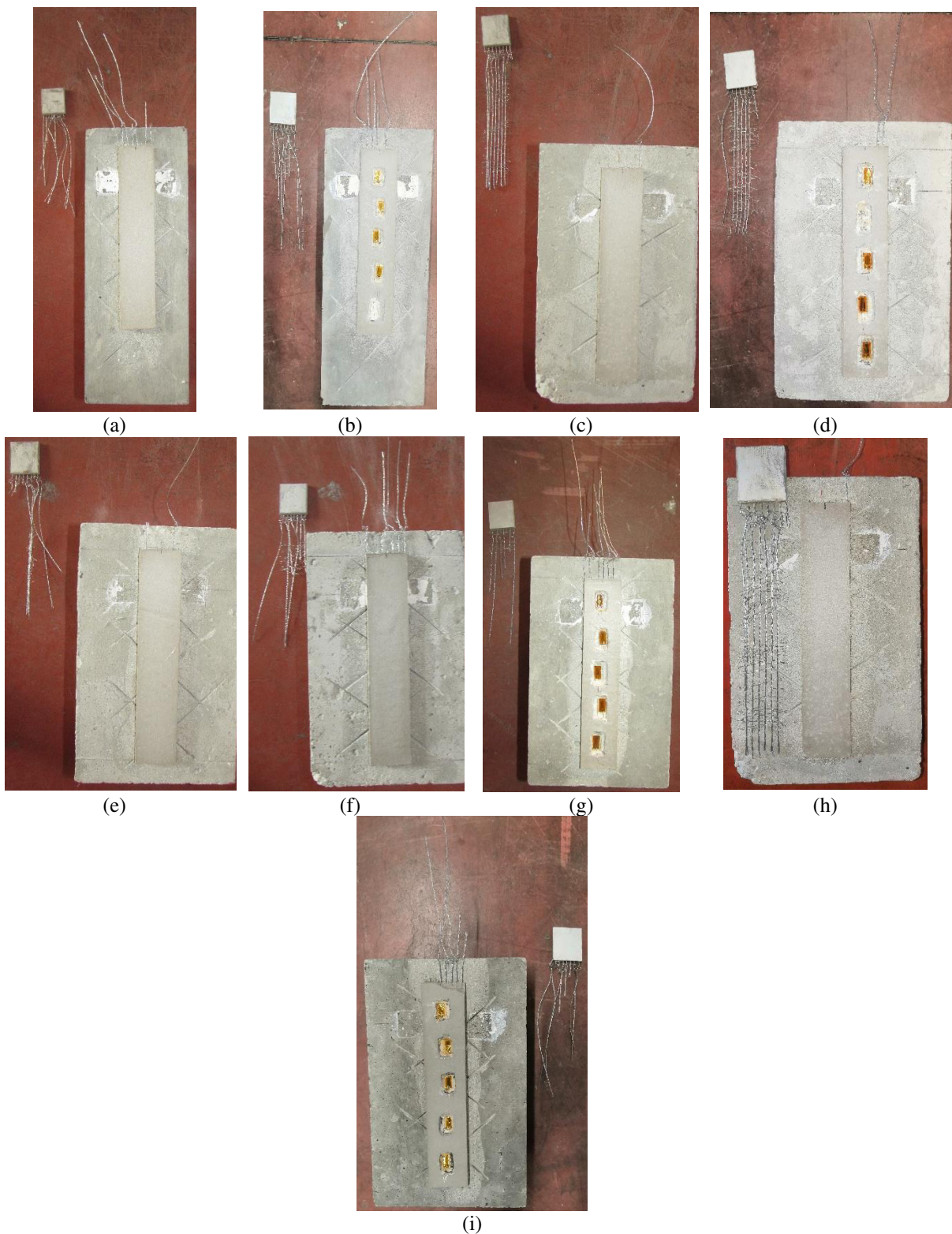
Figura 3.11 - Modalità di rottura: (a) DSC_GLV_BMN_1; (b) DSC_GLV_BMN_2; (c) DSC_GLV_BMN_4; (d) DSC_GLV_BMN_5; (e) DSC_GLV_BMN_6; (f) DSC_GLV_BMN_7; (g) DSC_GLV_BMN_8; (h) DSC_GLV_BMN_9; (i) DSC_GLV_BMN_11.
