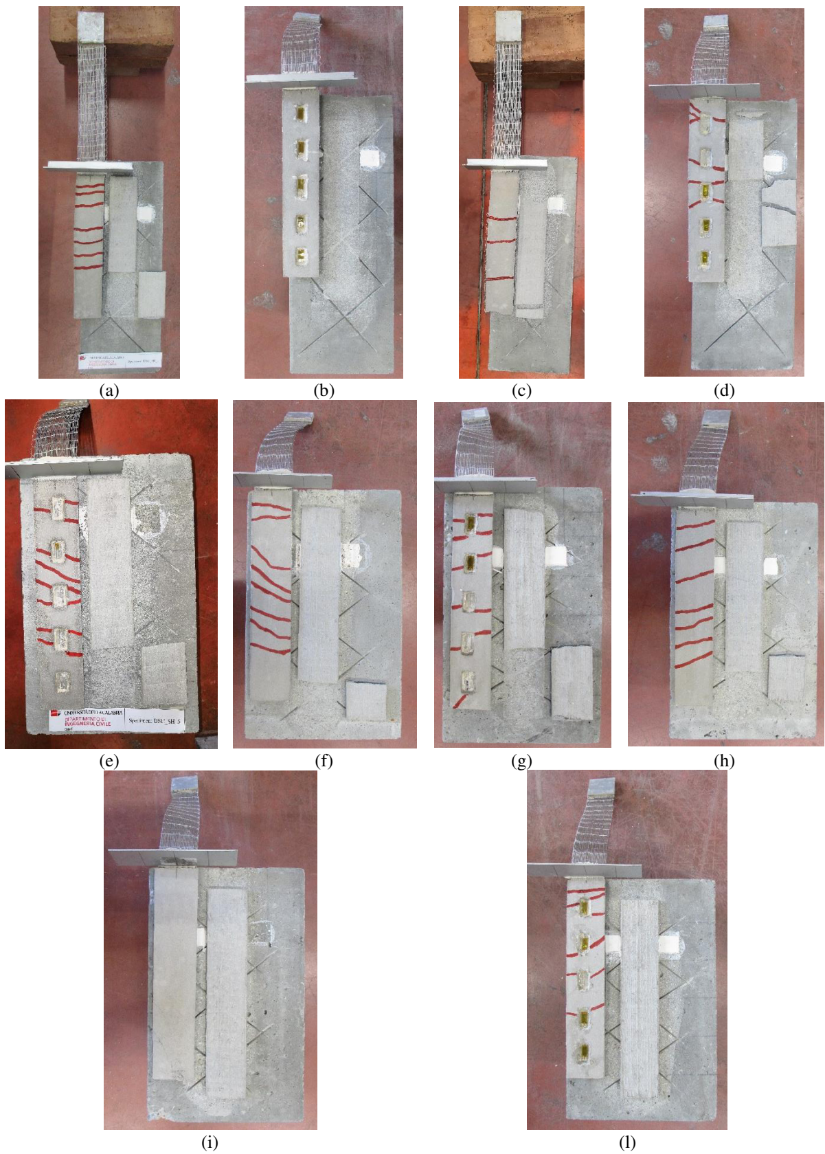
Figura 3.10 - Modalità di rottura: (a) DSC_SS_BMN_1; (b) DSC_SS_BMN_2; (c) DSC_SS_BMN_3; (d) DSC_SS_BMN_4; (e) DSC_SS_BMN_5; (f) DSC_SS_BMN_6; (g) DSC_SS_BMN_8; (h) DSC_SS_BMN_9; (i) DSC_SS_BMN_10; (l) DSC_SS_BMN_11.
