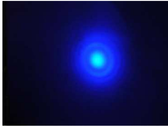
Figure 4.33: Spot of the laser emitted from the CLC cell on a screen placed at 10cm.
