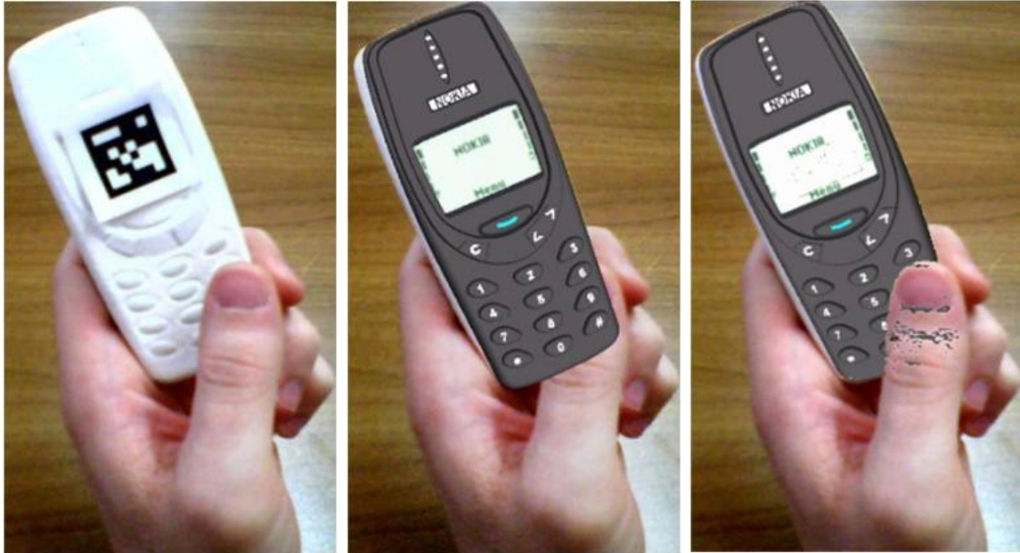
Figure 4.4: Occlusion Handling Details of Mixed Prototyping: the raw image from the HMD-camera (left) is composed with (right) and without (center) an occlusion handling strategy
