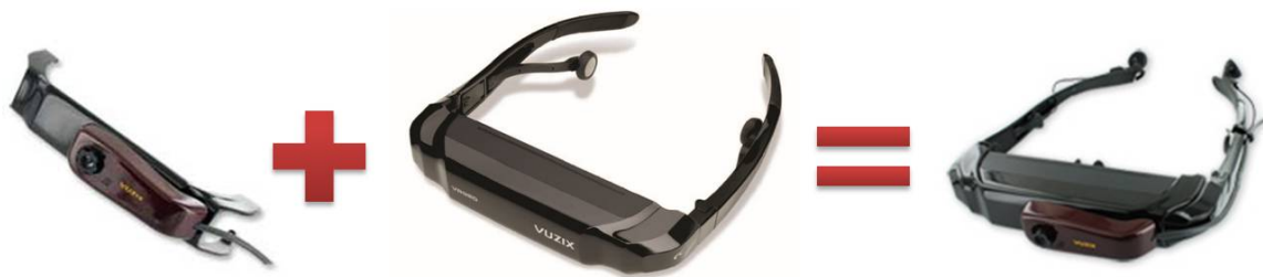
Figure 4.2: Vuzix HMD solution for AR: iWear CamAR bundled with iWear VR920
