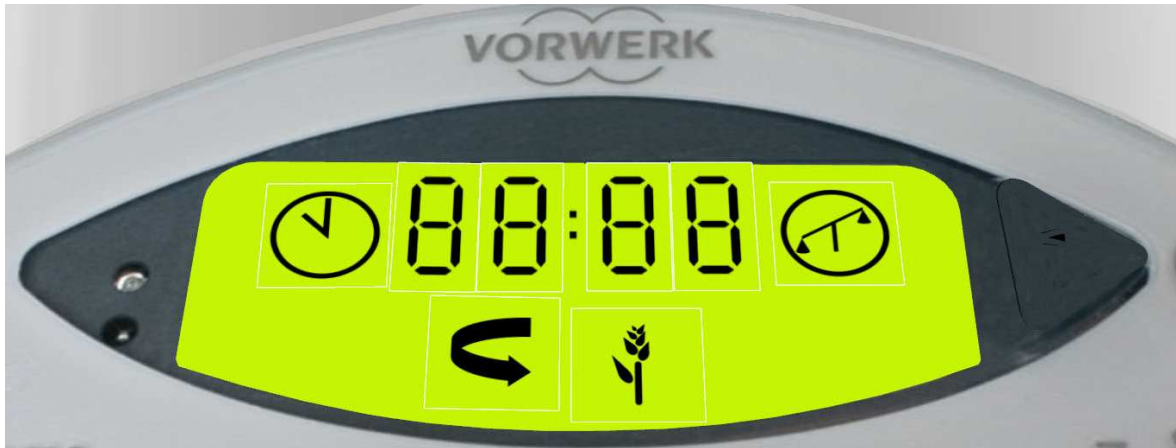
Figure 4.13: The display of the virtual product is made up of nine rectangular patches with different textures that are changed at run time by the simulator
