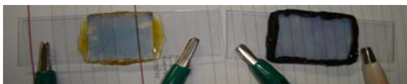
Fig. 2.45 ECD with ethyl viologen diperchlorate and ferrocene as catodic and anodic pair after 65000 electrical switching not sealed (on the left) and sealed with a butyl sealer(on the right).
