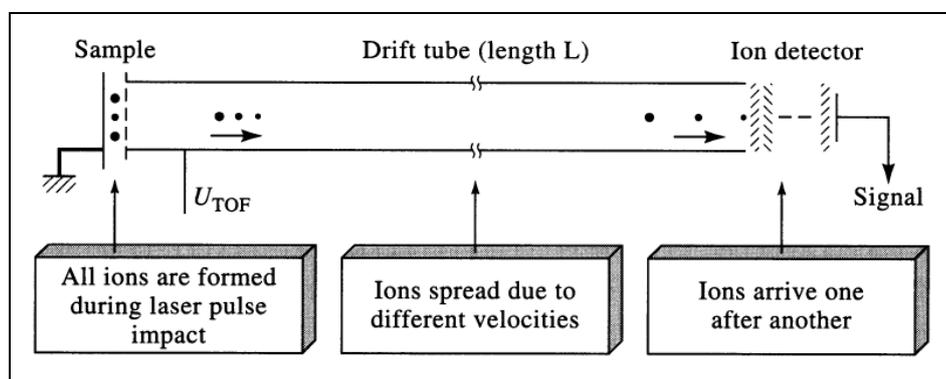
Figure 57. Schematic diagram of Time of flight mass spectrometer
