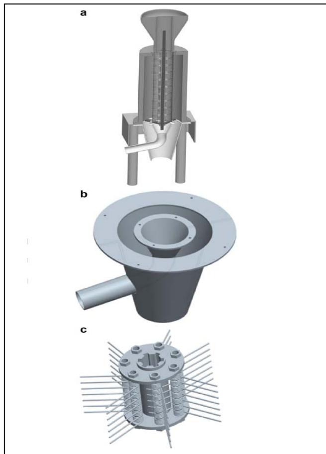
Figure 30. Sketch of the machine (a). The paste and stones collector at the bottom of the machine (b). The spring whips holder (c).
