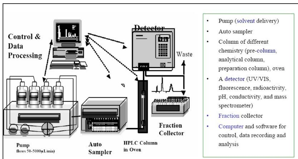
Figure 47. Schematic diagram of an high-performance liquid chromatograph.
