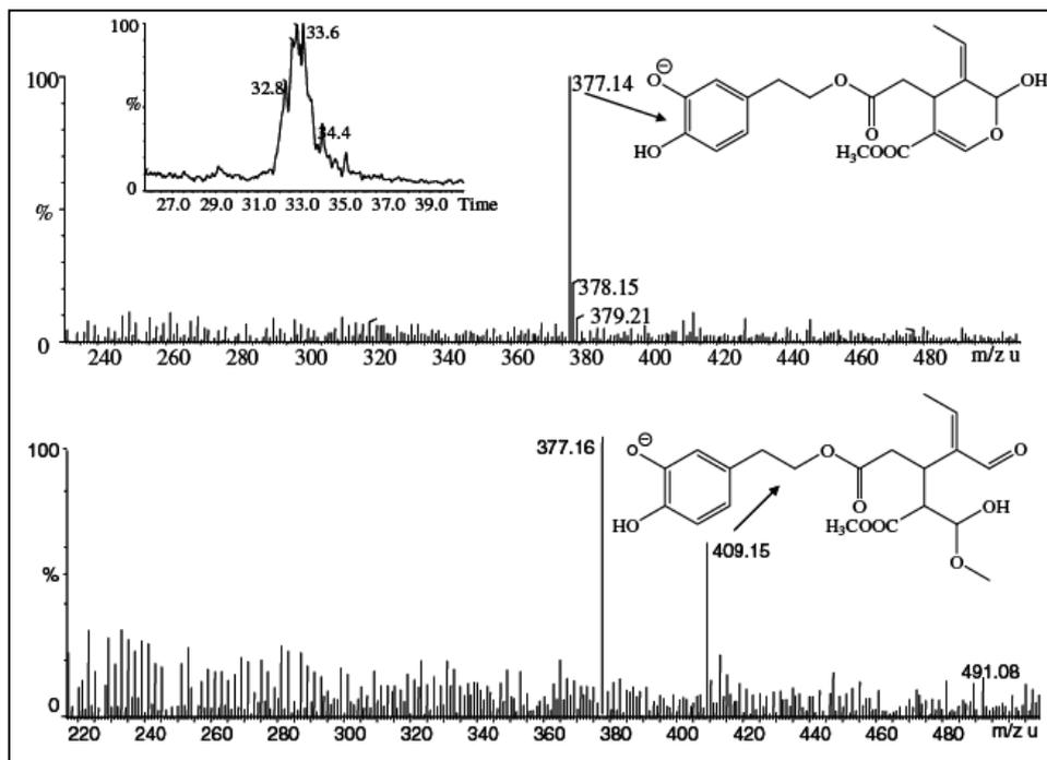
Figure 31. ESI-MS spectra taken directly from the solution containing OLP (1A) and the water extracts of Carolea pits after 60 min of incubation
