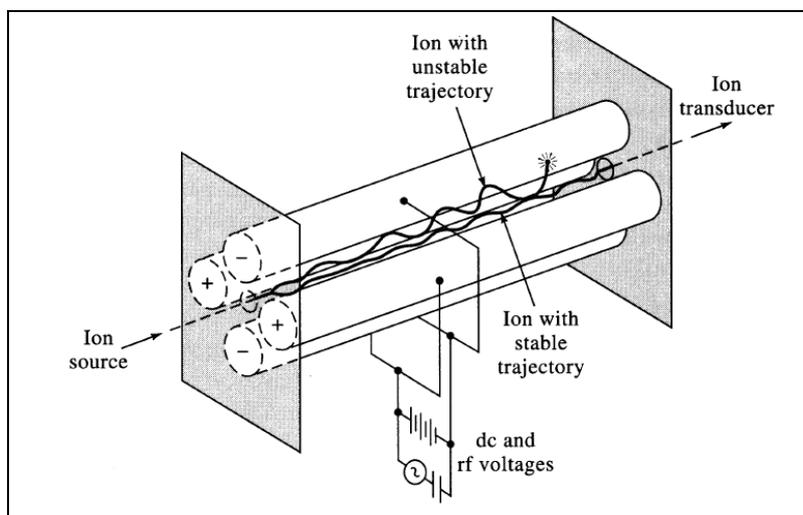
Figure 56. Schematic representation of Quadrupole Mass Analyzer
