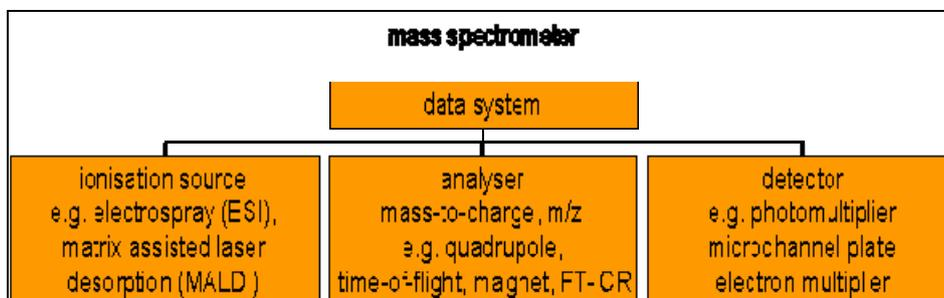
Figure 51. Simplified Schematic of a Mass Spectrometer
