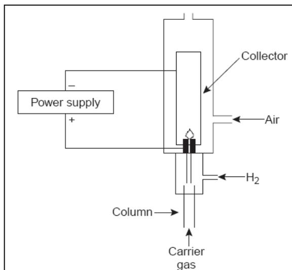
Figure 46. Schematic diagram of a FID detector for gaschromatography
