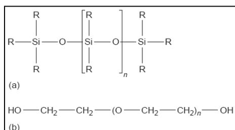
Figure 45. General structures of most common stationary phases for gas chromatography
