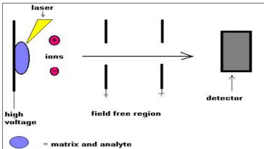
Figure 55. *Simplified schematic of MALDI-TOF mass spectrometry (linear mode)*
