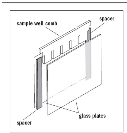
Figure 50. Diagram of vertical slab gel assembly ("sandwich"). The sides and bottom must be sealed liquid tight when the gel is cast.
