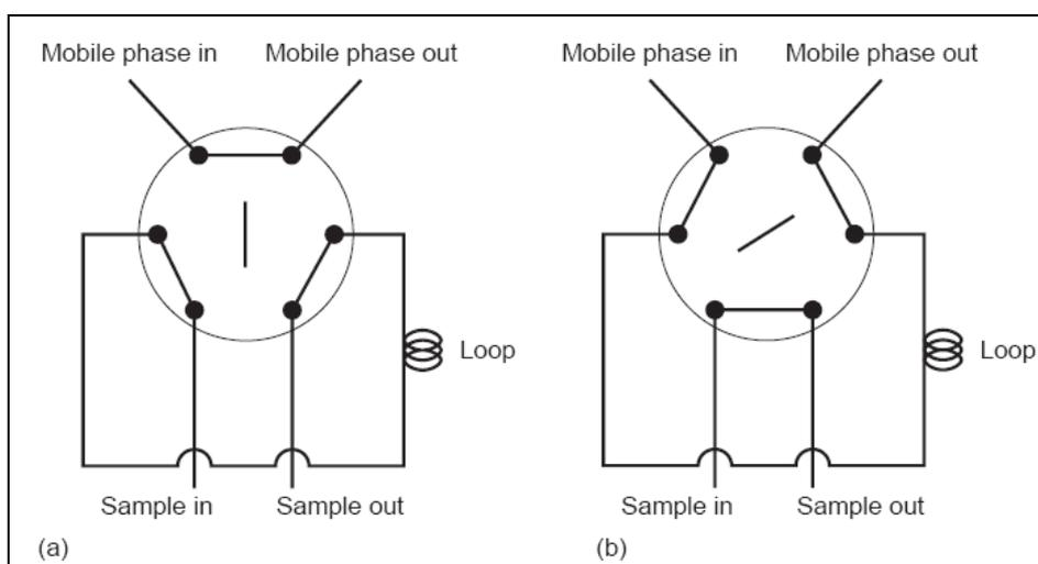
Figure 48. Schematic diagram of a loop injector in the (a) load and (b) inject positions.
