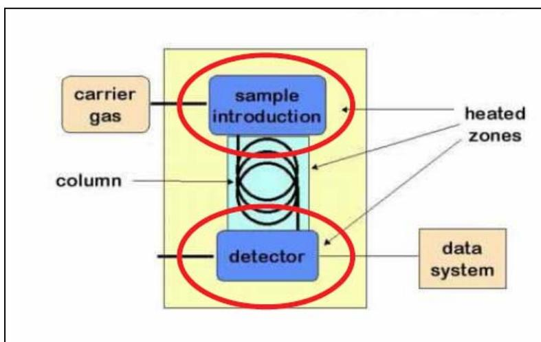
Figure 43. Schematic diagram of a typical gas chromatogram
