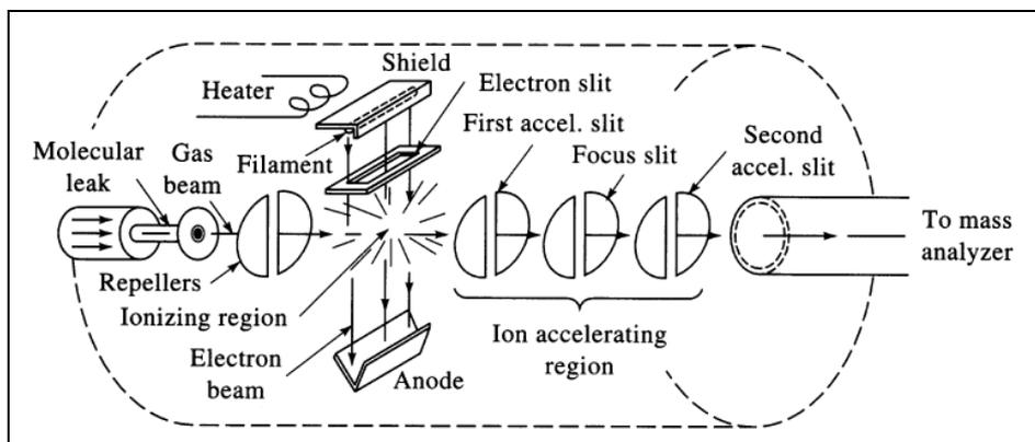
Figure 52. Schematic diagram of an electron impact source.
