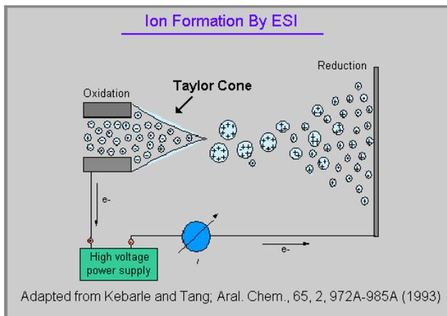
Figure 53. Schematic of an ESI interface
