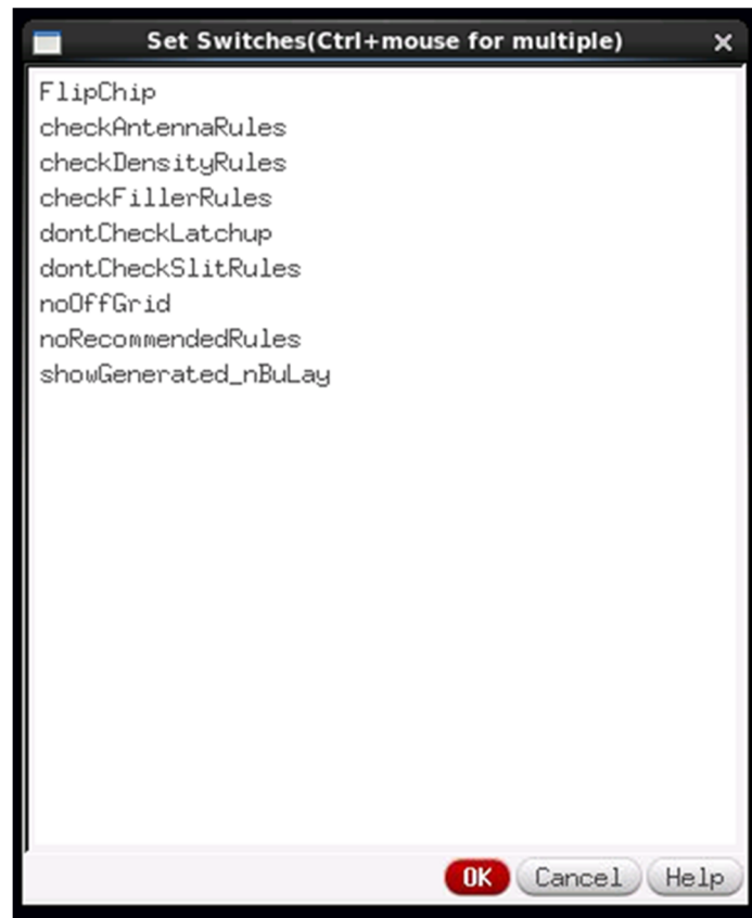
Figure A-7: DRC check switches in Assura.
