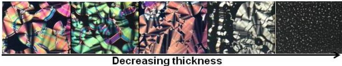
Figure 1.12: POM view (crossed polarizers,  $20\times$  Magnification) of a wedge cell made up with PB treated glass ( $40\mu\text{m}$  to  $0$ ), after 15 days from preparation, in which the thickness decreases from left to right as clearly visible from the picture, the colored ribbon textures change as optical retardation decreases.
