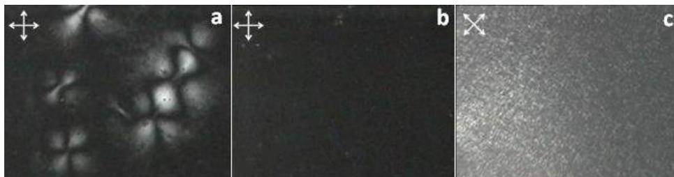
Figure 2.13: POM view of the cell filled with GMPNH4 using PB as alignment layer. All images are acquired using a  $20\times$  mag objective. (a) region with homeotropic anchoring and characteristic defects. (b-c) defect free region with a “modulation” of transmitted light intensity, indicating a tilt from normal alignment of the molecule.
