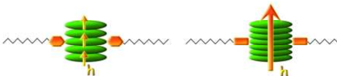
Figure 3.6: Schematic representation of the effect of the linkers on the stacking distance and on the charge carrier mobility in the columnar mesophases formed by mesogens with a triindole core.
