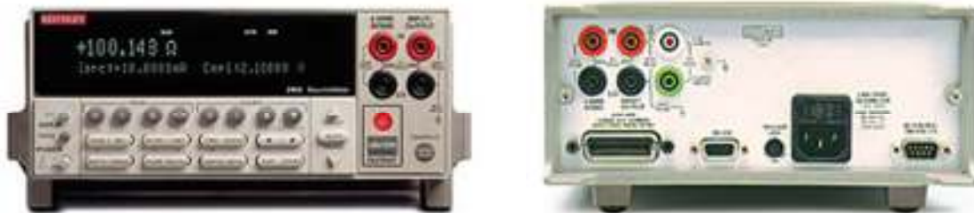
Figure 5.13. front and back view of the Keithley 2400 source measure unit.
