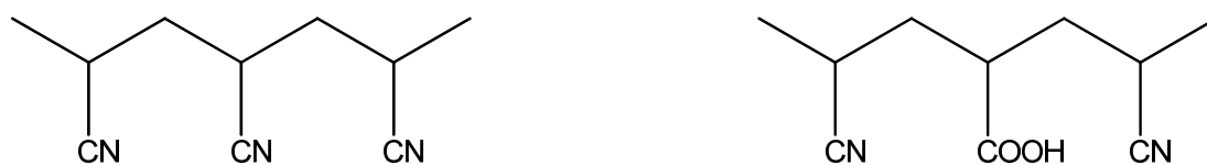
Figure 4.1 Chemical structure of models representing the polymeric chains used for the preparation of membranes.
