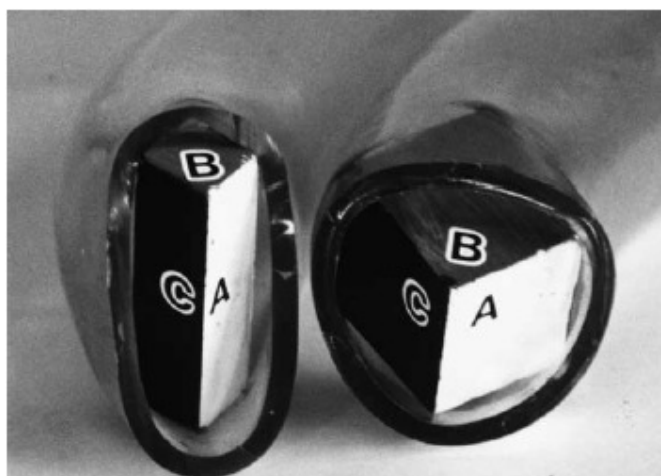
Figure II.33.: Growth model of the carbon microcoils: a) flat coils; b) circular coils [201]
