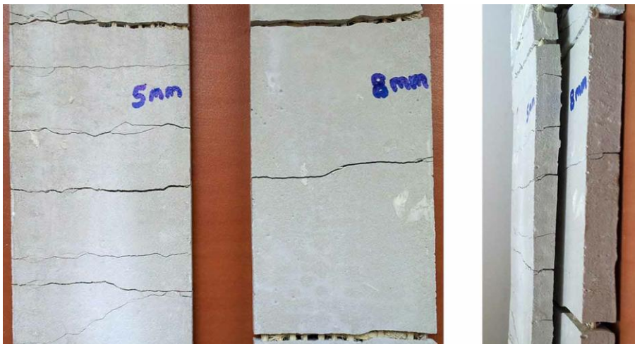
Fig. 3.11: Crack patterns of 5-mm-thick and 8-mm-thick sisal-FRCM composites: (a) front view; and (b) lateral view.
